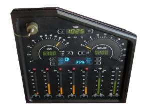
Driver's board is a control and signalling device dedicated to constant monitoring of operation parameters of selected systems of a vehicle, such as:
