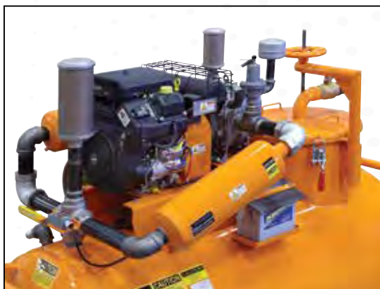
The "business side" of an electric start 25HP LP gas motor.
