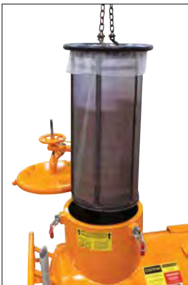
Chip basket captures chips and sludge from dirty coolant during cleaning.
