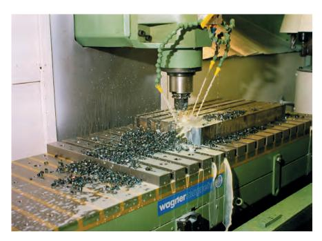
The electro permanent magnet clamping plate, type 1110V, with increased holding force is particularly suited for the milling of thick workpieces. The integrated and reinforced permanent magnetic clamping system generates a high depth effect to bridge air gaps in case of workpieces with uneven and rough surfaces.
