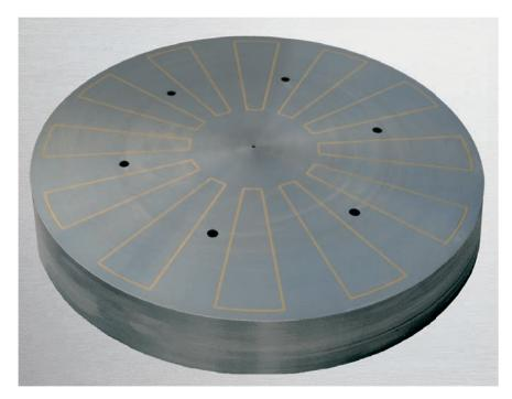
Electro-Permanent-Magnet-Clamping-Chucks, Type 1210, with radial pole spacing if several workpieces are clamped asymmetrically, they must cover at least two poles.
