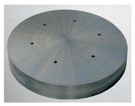
Electro-Permanent-Magnet-Clamping-Chuck Type 1210V with radial pole pitch and increased adhesive force are particularly suited for centrical clamping of rings, flanges, bearing housings and similar rotation-symmetric components
