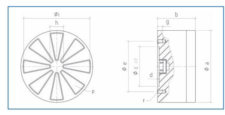
Electro-Permanent-Magnet-Clamping-Chuck Type 1210
