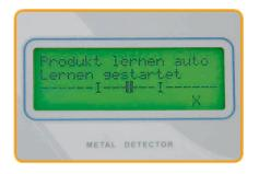
It is possible to store 50 different detector configurations. They can be invoked by using the text display. The standard controller provides english and german operation language. A third opration language can be pre-installed by Wagner or can be loaded in field.
